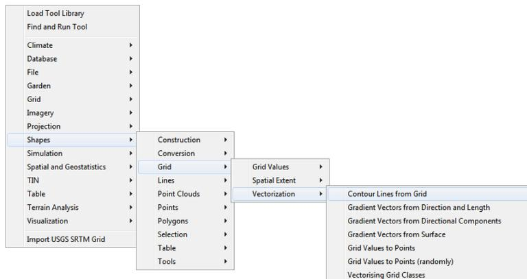
Set the grid system and contour interval in the **Contour Lines from Grid** window:
